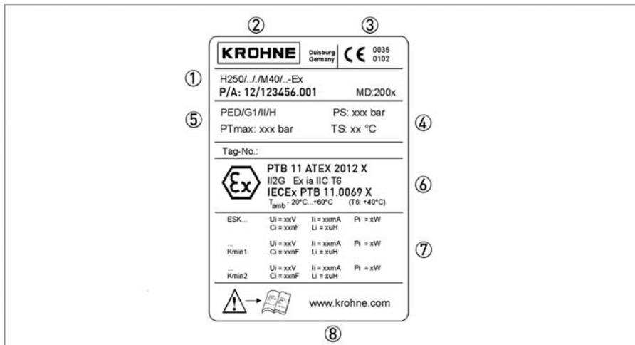
Figure 2-2: Nameplate on the indicator
