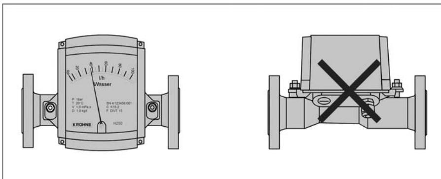
In order to comply with thermal parameters and measuring accuracy, H250H flowmeters for horizontal installation are to be installed in the pipeline so that the display is located on the side of the measuring tube. The maximum medium and ambient temperatures indicated as well as the measuring accuracy are based on lateral installation of the display.
