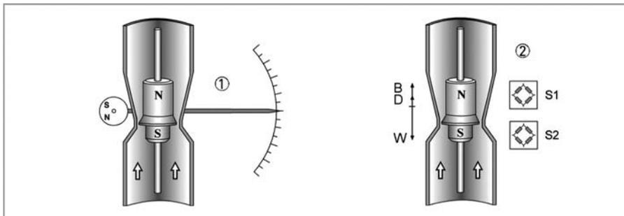
Figure 1-1: Operating principle
