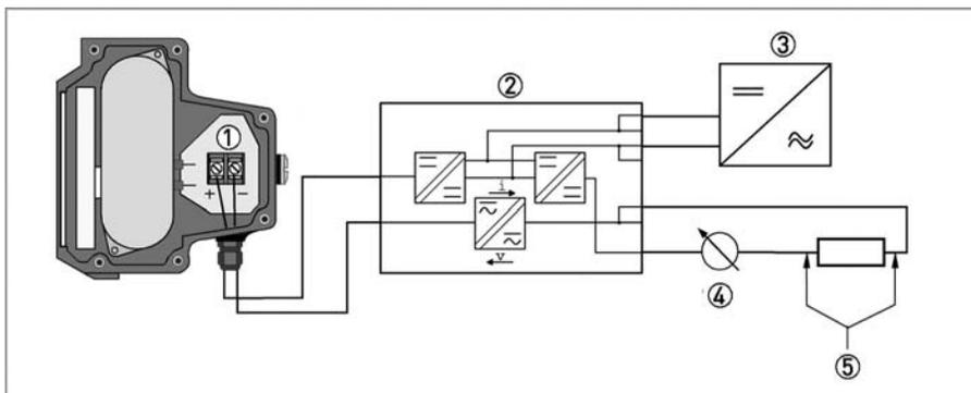
Figure 4-3: Electrical connection M8EG with electrical isolation
