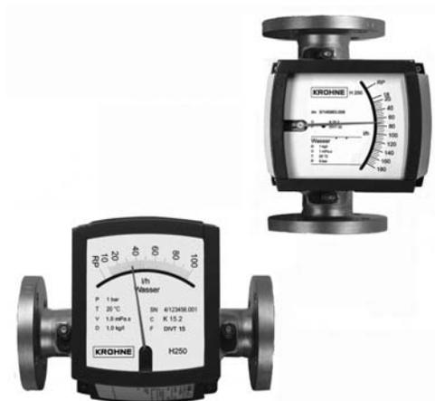
Variable area flowmeters typically feature a vertically positioned measuring cone through which the medium flows from bottom to top, lifting a float against the weight.
