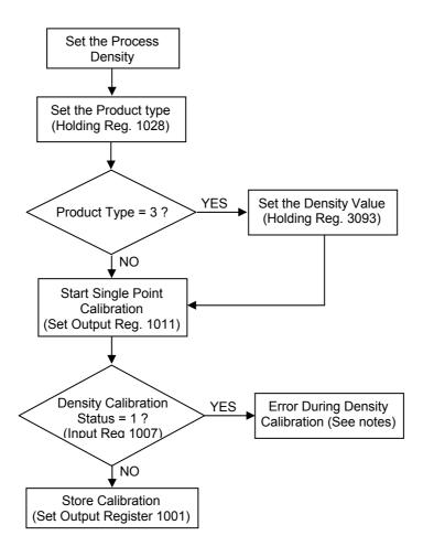
An error flag is set in the "Density Calibration" input status register when the measured tube frequency does not correlate with the value/product type of the calibration density entered by the user (e.g. if the user requests a calibration of the "Air" type when the tube is full of process fluid.)
