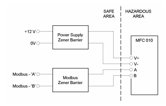
The Zener barrier devices must be installed in an EMI shielded enclosure and the cable screen(s) kept intact right up to the barrier terminals as far as is practical. The cable screen(s) should be terminated to the enclosure, chassis Earth connection, and kept <u>SEPARATE</u> from the intrinsically safe Earth connections of the Barrier devices. The user <u>MUST</u> adhere to the barrier manufacturer's instructions for connecting the intrinsically safe Earth connection to the barrier devices.
