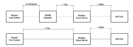
Where the distance from the barrier device to the MFC010 is less than 10m, two barrier devices may be connected in parallel to the "Master" host system, or the repeater if one is being used, refer to the diagram below. The overall cable length from the Host/repeater to the barrier devices must still be less than 10m as described previously. If more than two devices are required to be connected then a dedicated repeater should be used for each.
