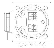
**NB**. When using foil-screened cable, the integral drain wire should not be relied upon to provide a secure ground connection to the foil screen. The foil screen must be terminated directly to a robust Earth point at both ends of the cable, on the MFC010 using the EMC cable gland provided.
