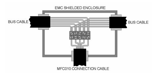
If the Bus does not provide a suitable power supply for the MFC010, a separate suitable power supply connection should be made at this point.
