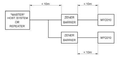
Each MFC010 <u>MUST</u> have its own dedicated barrier interface; they <u>MUST NOT</u> be connected in parallel on the hazardous area side of the system.
