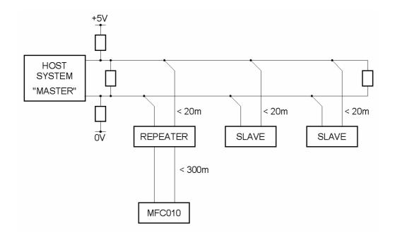
Because the connection to the bus requires exposing the signal wires, the connection to the main bus should be made within a suitable EMI shielded enclosure. This connection should include the "Common" signal connection, the power supply connection (if a suitable one is provided by the bus), and the drain wire when available. Each of the cable screens must be properly terminated to the enclosure by means of appropriate EMC cable glands. For example:
