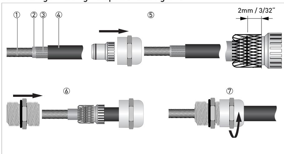
Figure 3-12: Connecting the shield within the cable gland
