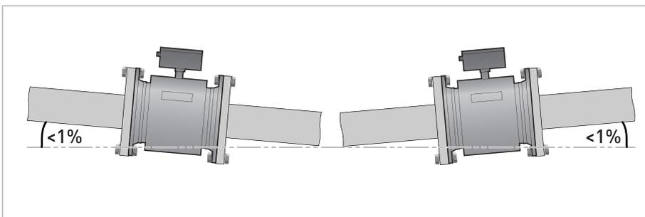
Figure 2-9: Recommended slope
