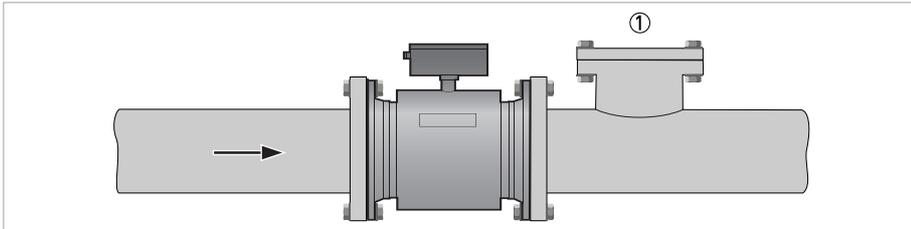
Figure 2-11: Option for cleaning of flow sensor
