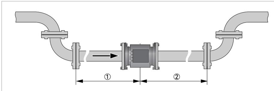
Figure 2-3: Recommended inlet and outlet sections, top view
