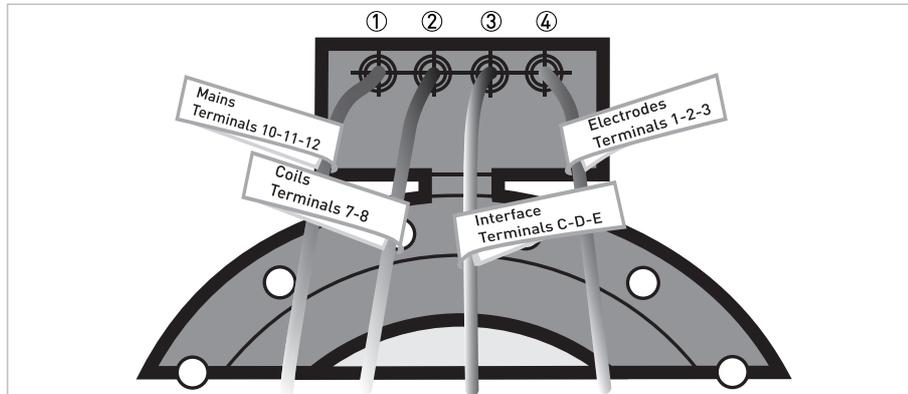
Figure 3-3: Labeled cables for IP 68 versions
