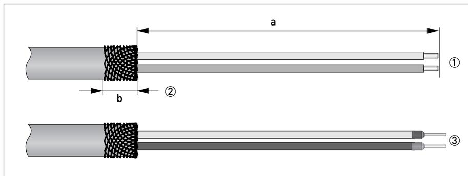
Figure 3-8: Preparation of field current cable C
