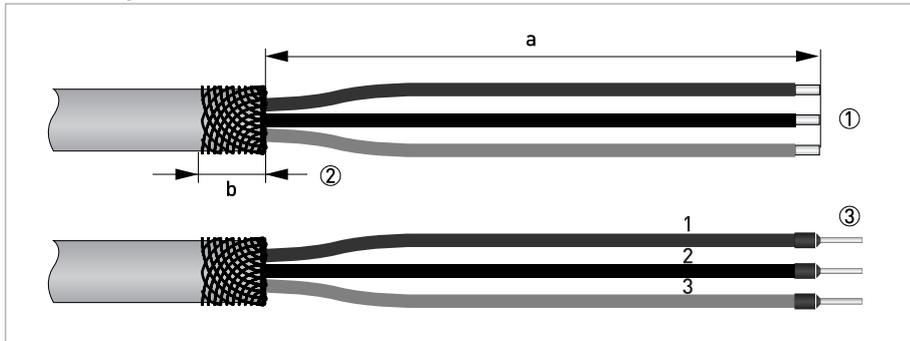
Figure 3-11: Preparing the interface cable
