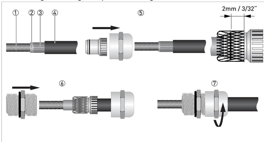
Figure 3-10: Connecting the shield within the cable gland
