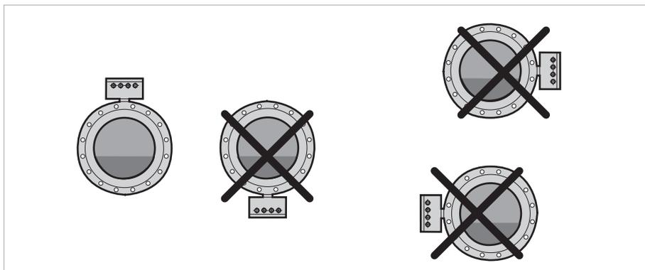
Figure 2-4: Mounting position
