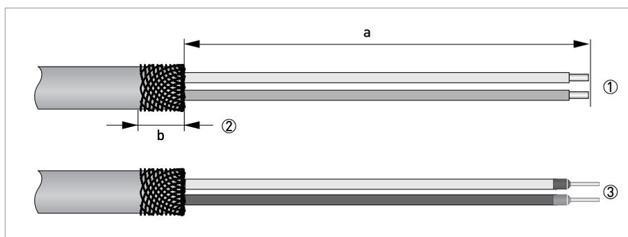
Figure 4-8: Preparation of field current cable C
