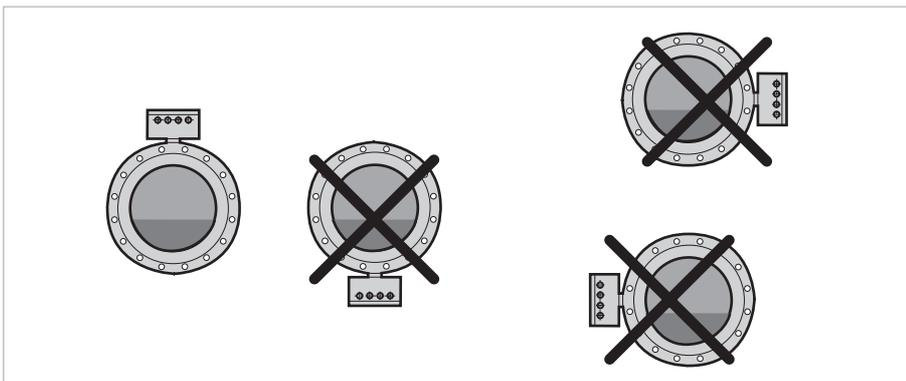
Figure 3-2: Mounting position
