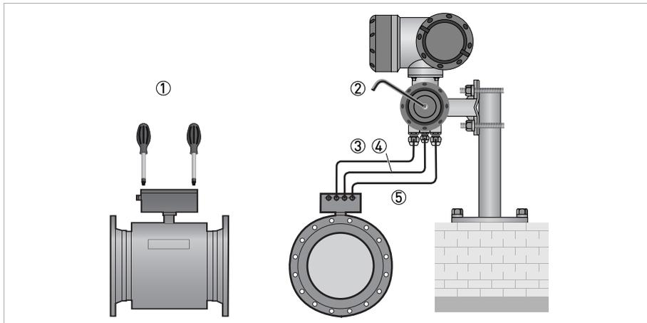
Figure 4-1: Electrical connection
