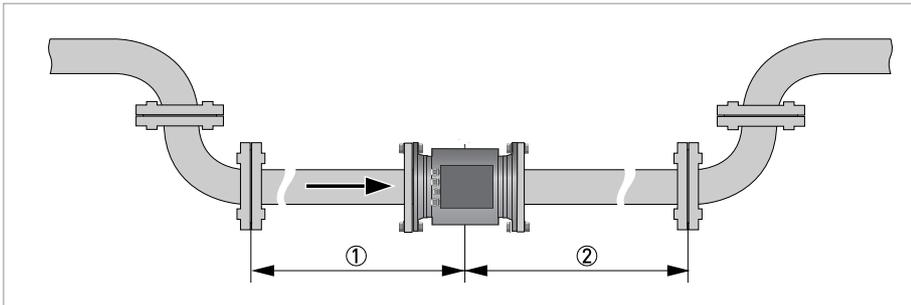
Figure 3-1: Recommended inlet and outlet sections, top view
