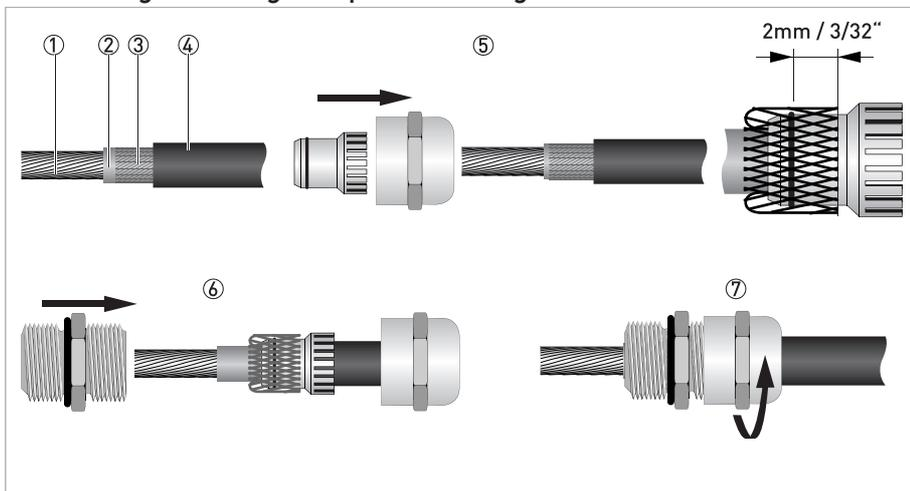
Figure 4-12: Connecting the shield within the cable gland
