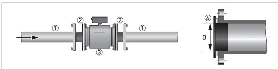
Figure 3-10: Grounding with grounding rings
