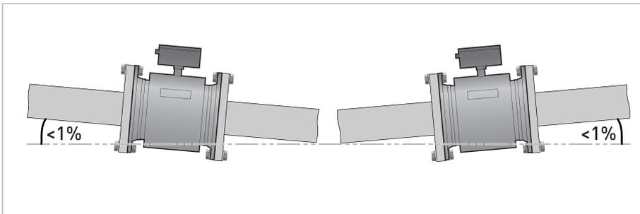
Figure 3-7: Recommended slope
