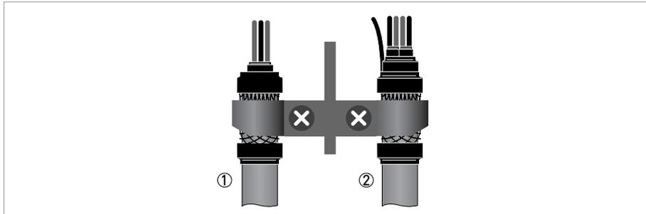
Figure 4-9: Clamping of shields
