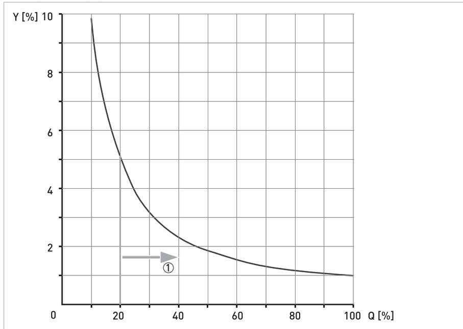
Figure 2-2: Maximum measuring error of measured value.
