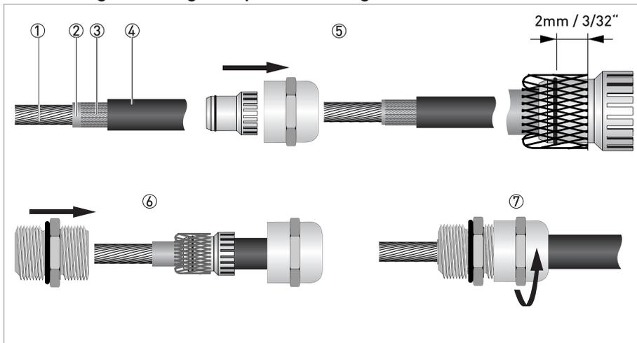
Figure 4-10: Connecting the shield within the cable gland
