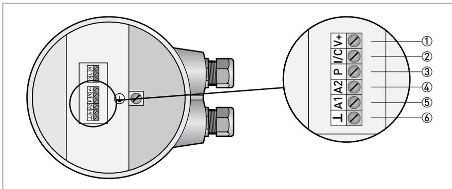
Figure 4-3: Terminals for standard instrument.
