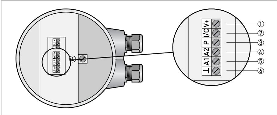
Figure 4-5: Terminals for non Ex HiPower instrument.
