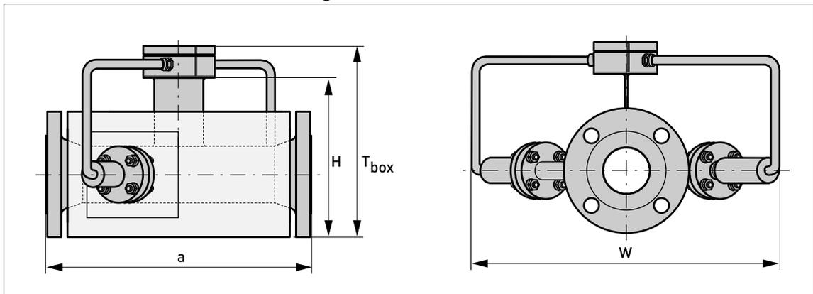
Front and side view  $\geq$ DN100 (dual beam construction)
