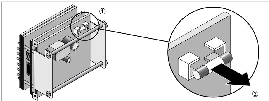
Figure 7-5: Removing fuse
