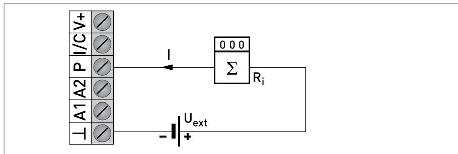
Figure 4-13: Pulse output (passive)
