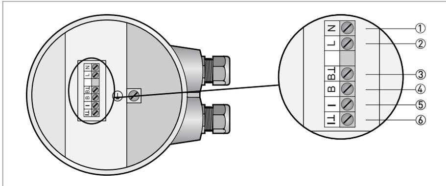
Figure 4-8: Terminals for instrument with Ex-i (Modis)
