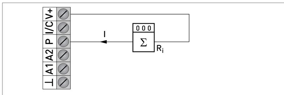
Figure 4-12: Pulse output (active)
