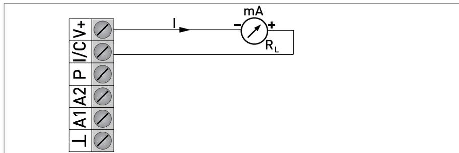
Figure 4-10: Current output (active)
