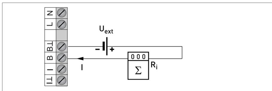
Figure 4-14: Pulse output (passive) for Ex-i Modis
