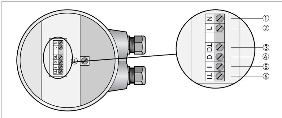
Figure 4-9: Terminals for Ex-i (Modis) version with Profibus PA
