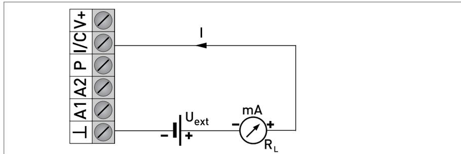
Figure 4-11: Current output (passive)
