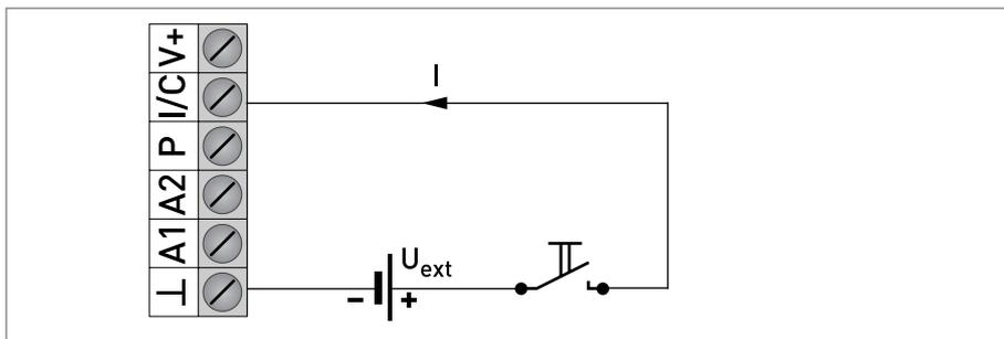
Figure 4-16: Digital input (passive)
