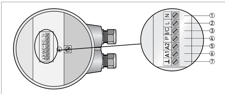
Figure 4-6: Terminals for Ex standard instrument
