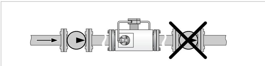
Figure 3-7: Install pump upstream of flowmeter.
