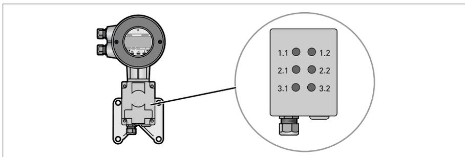
Figure 4-3: Connection of the sensor cables, converter side
