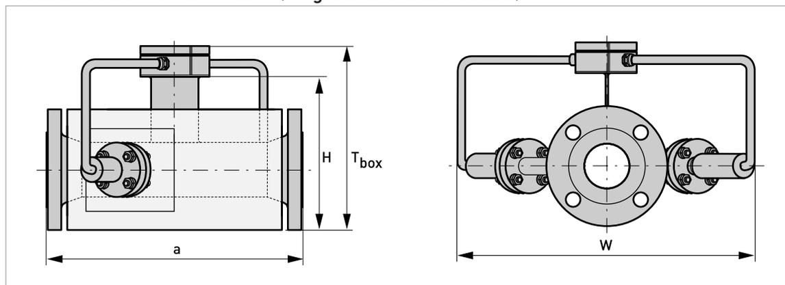
Front and side view  $\geq$ DN100 (dual beam construction)
