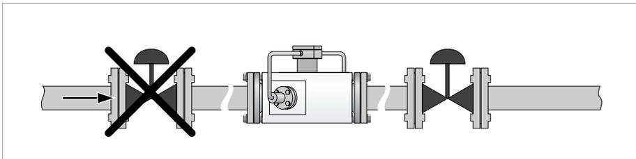
Figure 3-6: Install control valve downstream of the flow meter.
