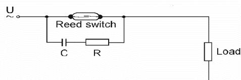
Protection with an RC circuit for a.c. current and inductive load.
